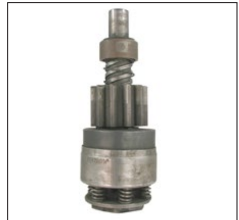
William Weldon rebuilt these inertia friction drives for Bendix, to Bendix specifications over 50 years ago.
